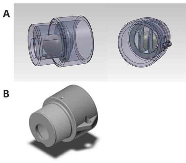
**Figure 2.** The Shikani speaking valve port at the 12 o'clock position. The small, half-moon-shaped notch on the front is positioned at 12 o'clock (the valve-up or bias-open configuration).
