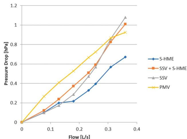
airflow (L/s). The results indicate that there was no statistically significant difference between the devices and that in-line use of the SSV + S-HME does not add significant  $R_{\text{airflow}}$  beyond that of the SSV alone or the PMV alone. The PMV alone showed a trend toward a higher  $R_{\text{airflow}}$ ; however, the difference did not achieve statistical significance. The ANOVA results are shown in Table 2.
