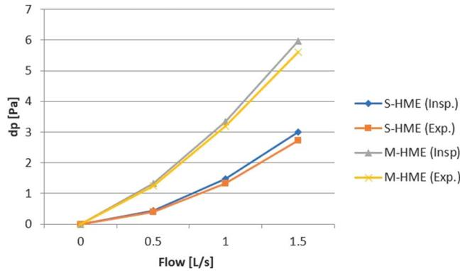
HME before and after each series of tests. ML was compared between the S-HME (turbulent airflow) and M-HME (linear airflow).
